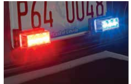
IPX312-4 and IPX312-3 mounted with IPX-LPF1 bracket on license plate, on Ford Police Interceptor Sedan
